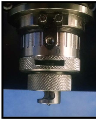
Figure 4: Micrometer after drill has been set to proper depth.
