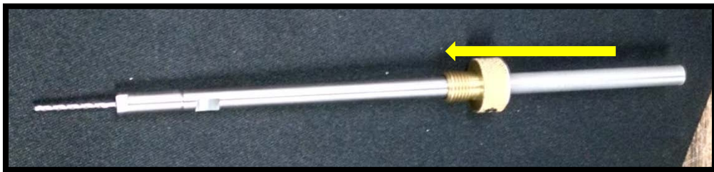
Figure 2: Adjust brass piece so drill will not extend past nose cone when inserted into spindle.
