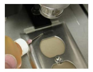
**Step 4/Photo 4:** Send the job to the engraver. Use a very slow feed rate and high RPMs when deep-engraving into stainless steel. Here, we used an XY and Z feed rate of .1 inches per second and a spindle speed of 18,000 RPMs. Clean debris off the material using a brush, vacuum, or compressed air.
