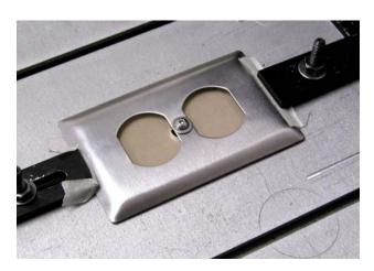
**Step 2/Photo 2:** For this example, we set the Home position in the center of the area to be engraved to minimize potential variances in depth. We then set the surface of the tool on the material.
