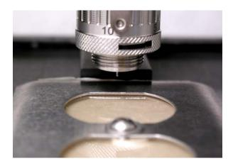
**Step 3/Photo 3:** When deep-engraving into hard metals, always use a coolant. Here, we used a few drops of cutting oil and smeared it over the area to be engraved. Another great option is to use a Unist lubrication system, which applies a steady amount of a vegetable-based coolant onto the surface. Vision now offers Unist Systems as an option for their CNC routers.
