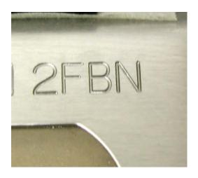
**Step 5/Photos 5, 6 and 7 (Optional):** To enhance the text and increase contrast, you can flood the engraved area with paint and let dry for a minute. Put a dab of alcohol on a cloth. Wrap the cloth around something with a rigid edge (such as a piece of scrap metal or plastic) and wipe back and forth removing any excess paint.
