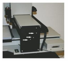
Step 2 - Remove screws with allen tool
