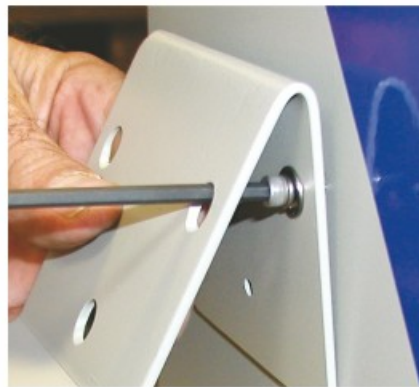
Step 2 - Secure Pendant Holder to machine with screws
