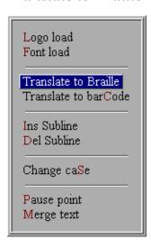
This feature will change the current line of text into Grade II Braille. It will translate the text, change the font to the Braille font and change the letter height to the standard Braille letter height.
