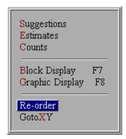
This feature will allow you to change the engraving order of your lines in your layout. It is often used to reduce the amount of cutter up travel or to minimize the need to change the cutter during the job.
