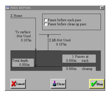
**To surface:** This value is ignored when using the Vision Serial Controller or the VE-810 Engraver. The surface is set on the controller and in the VE-810.
