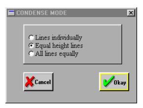
**Condensation** is how tight the text is compressed to make it fit in an area so it doesn't go off of the sign blank. It is measured in a percentage. Ex. A condensation of 80 percent would condense or compress the text by 80 percent and a condensation of 120 percent would stretch the text to 120 percent. A "normal" condensation is 100 percent.
