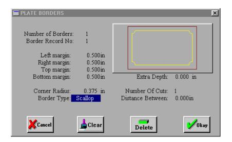
**Number of Borders**: This is the total number of borders on the plate. Vision allows you to have up to eight borders on a single plate. You can make a sign look unique by using multiple borders.
