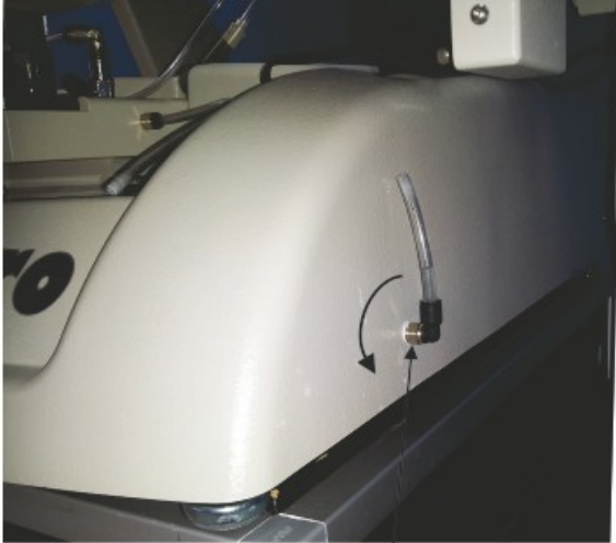
Water Level Indicator Fitting Rotate in Direction Shown to Drain System
