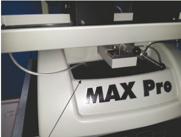
Water Reservoir Cover
