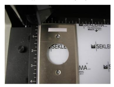
Move the spindle using the X, Y and Z buttons on the engraver, so that the tip of the cutter is directly over the upper left hand corner of the engraving area. The pictures below show the spindle/cutter tip correctly positioned in the upper left corner of the engraving area.
