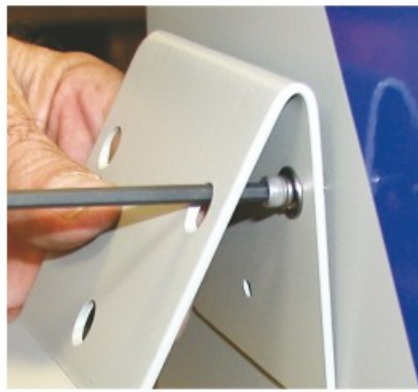
Step 2 - Secure Pendant Holder to machine with screws
