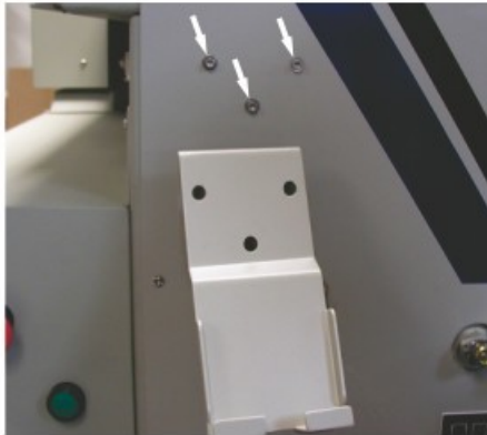
Step 1 - Locate and remove the three mounting screws
