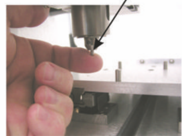
Install new cutter until it stops in top position, then tighten set screw
