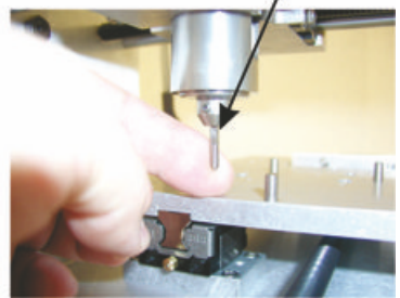
Install new cutter until it stops in top position, then tighten set screw
